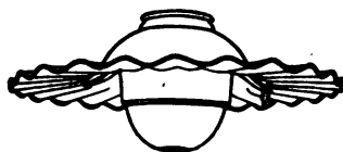
18-INCH RADIAL BOWL REFLECTOR WITH 6 1/2-INCH HOLOPHANE SKIRTED REFRACTOR FOR 100 AND 150-WATT TYPE C MULTIPLE LAMPS
